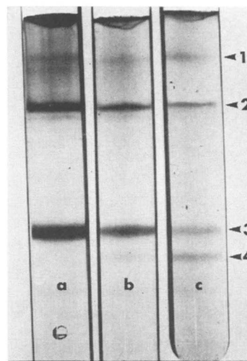
FIG. 4. Acrylamide electrophoresis in 8 M urea at pH 8.9 of totally delipidated liposomes and VLDL. Gels a and c are totally delipidated liposomes and VLDL, respectively. In gel b, liposomes and VLDL were mixed prior to delipidation. Direction of migration is from top to bottom. Concentration of acrylamide was 4%. Gels were stained for protein with Coomassie brilliant blue. The amount of liposomal material used is greater than the amount of VLDL in order to emphasize the points of comigration.
